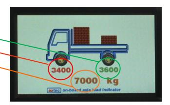
In addition to the displayed load values, Axtec OnBoard gives a graphical representation of the load and load distribution, using a stack of bricks per axle. As the load increases, the stack gets higher until, when the vehicle is overloaded, the stack is higher than roof level
